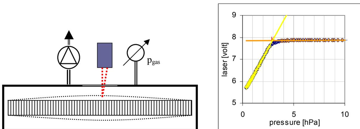
Fig. 3: Left: Principle of the internal pressure detection in a VIP (see text). Right: Evaluation of a distance-pressure diagram to determine the "critical" pressure (beginning of displacement of the barrier film).
