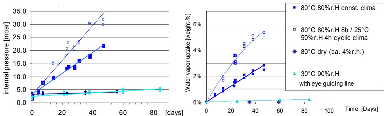
Fig. 4: Increase of internal pressure (left) and moisture content (right) in "small" VIP at elevated temperature / humidity. The measurements were done at room temperature after cooling down the samples for about 1 h. Discussion: see text.
