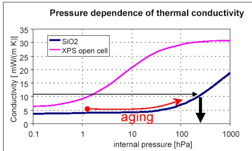
Fig. 2: Thermal conductivity of two core materials as a function of the gas pressure in the pores.
