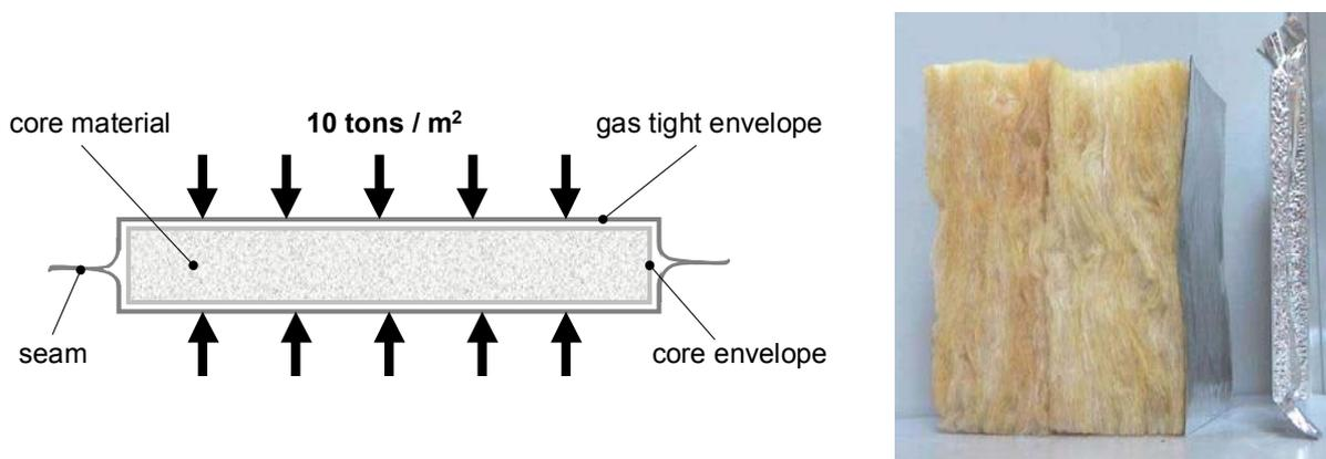
*Fig. 1: Schematic cross section through a VIP (left), comparison of a conventional mineral wool insulation board and a VIP with equal thermal resistance (right).*
