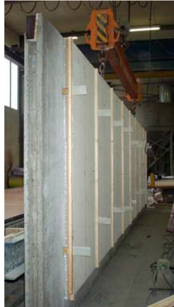
Figure 61: Left: Intended design for the prefabricated wall elements. An average U-value of 0.15 \text{ W}/(\text{m}^2\cdot\text{K}) is achieved with a total thickness of only 27 cm. Right: Photo of a prefabricated wall element
