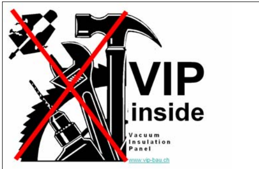
Figure 5: Draft sketch for an adhesive warning label to mark VIP panels and building components containing VIP
