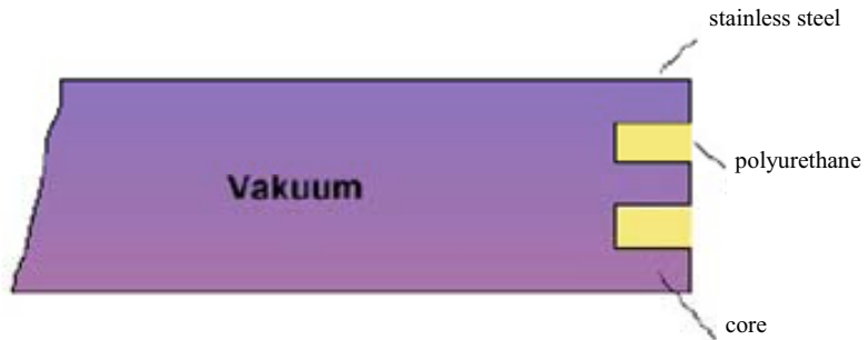
Figure 14: Section through a VIP. Sketch of the serpentine construction
