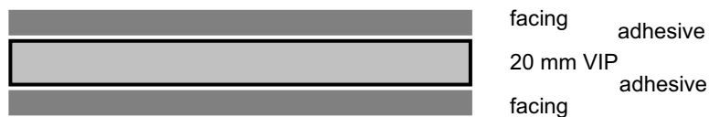
Figure 17: The layout of sandwich panels
