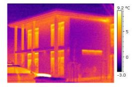
Kind of insulation: Facade insulation with vacuum insulation panels
